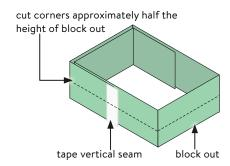
Make cuts in each of the four corners approximately half the height of the Block Out. Remove formed Block Out membrane form, flip over and replace on Block Out spreading flaps to horizontal position.
